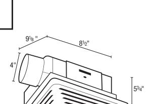
Acceptable for use over tub or shower when installed in a GFCI protected branch circuit.
