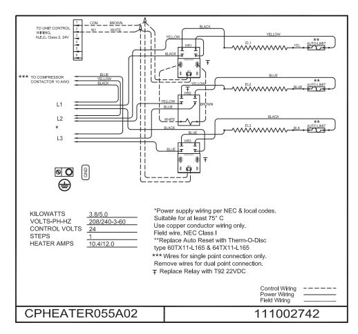
Fig. 18 - CPHEATER055A02 Wiring Diagram
