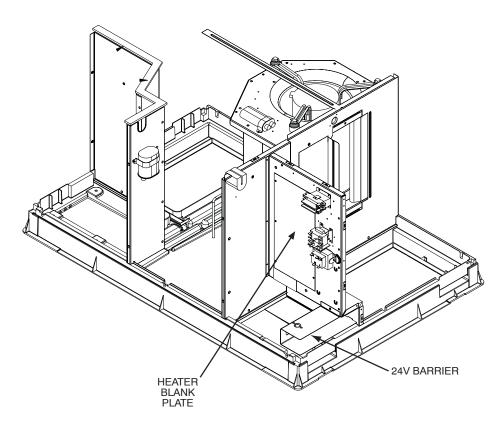
Fig. 3 - Heater Blank Plate Location
