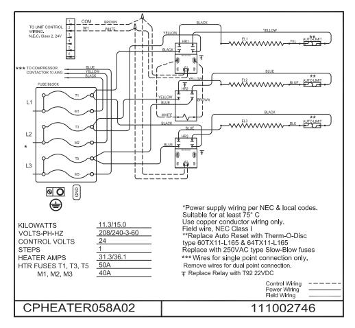
Fig. 21 - CPHEATER058A02 Wiring Diagram
