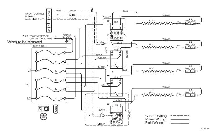
Fig. 4 - Wiring Diagram Example for Fused Heater
