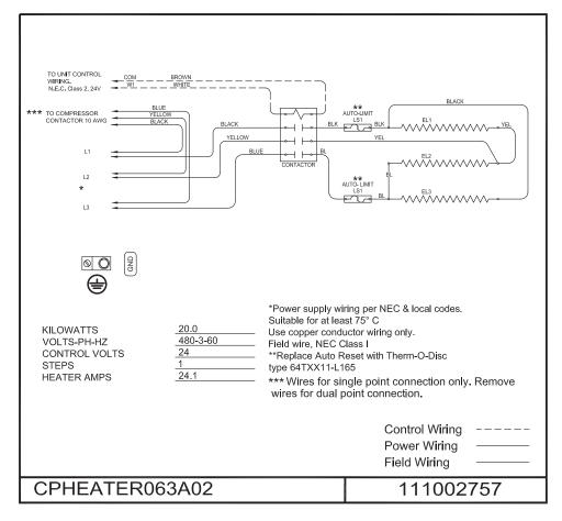
Fig. 25 - CPHEATER063A02 Wiring Diagram
