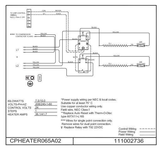
Fig. 27 - CPHEATER065A02 Wiring Diagram
