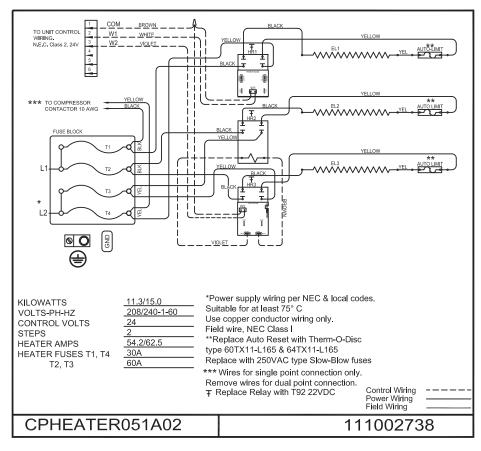
Fig. 14 - CPHEATER051A02 Wiring Diagram
