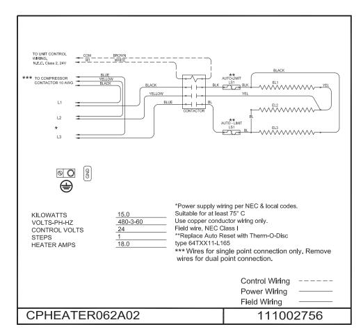
Fig. 24 - CPHEATER062A02 Wiring Diagram
