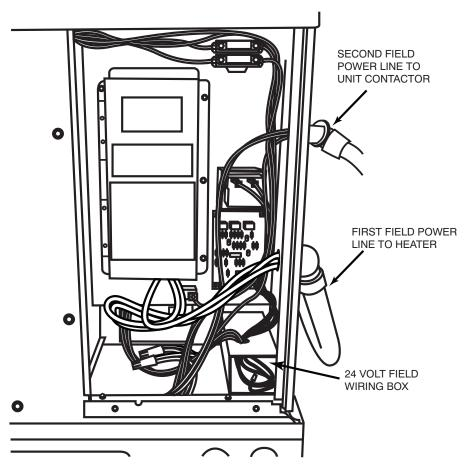
Fig. 8 - Dual Point Connections for Fused Heater
