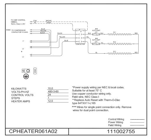
Fig. 23 - CPHEATER061A02 Wiring Diagram
