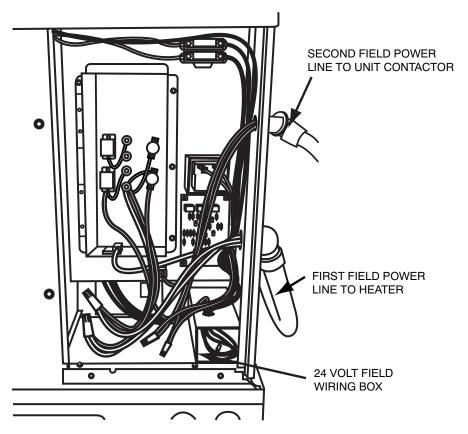
Fig. 9 - Dual Point Connection for Non-Fused Heater
