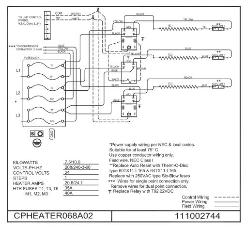
Fig. 29 - CPHEATER068A02 Wiring Diagram
