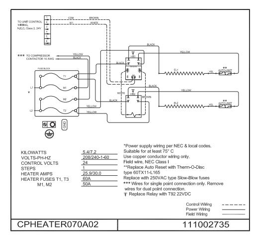
Fig. 31 - CPHEATER070A02 Wiring Diagram
