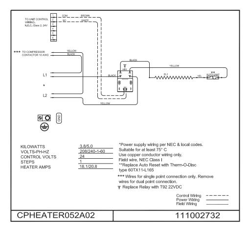
Fig. 15 - CPHEATER052A02 Wiring Diagram
