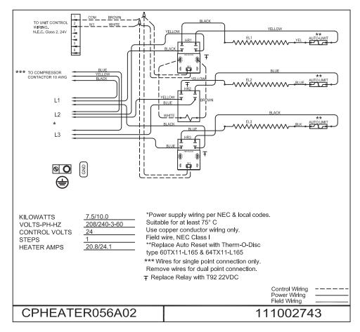
Fig. 19 - CPHEATER056A02 Wiring Diagram
