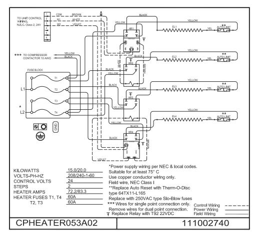
Fig. 16 - CPHEATER053A02 Wiring Diagram
