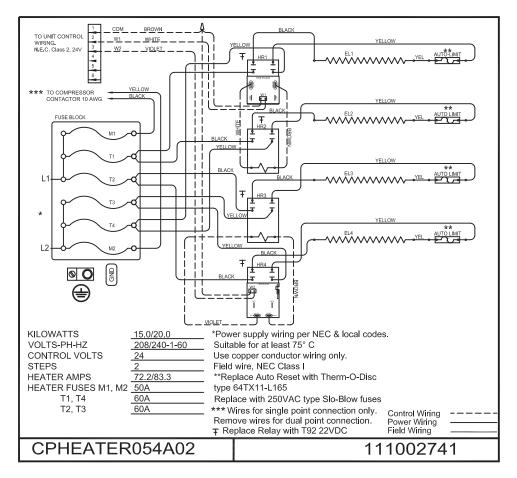
Fig. 17 - CPHEATER054A02 Wiring Diagram
