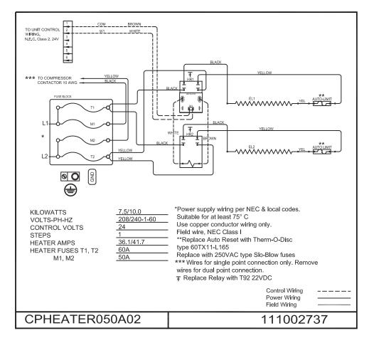
Fig. 13 - CPHEATER050A02 Wiring Diagram
