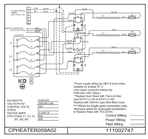
Fig. 22 - CPHEATER059A02 Wiring Diagram
