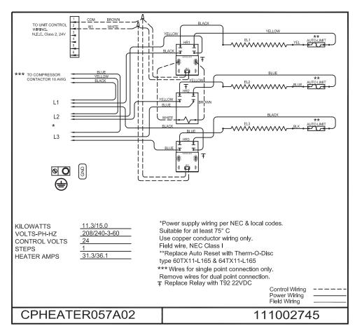
Fig. 20 - CPHEATER057A02 Wiring Diagram
