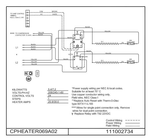
Fig. 30 - CPHEATER069A02 Wiring Diagram
