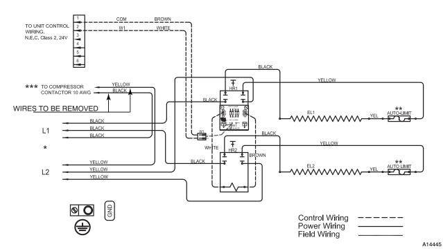
Fig. 5 - Wiring Diagram Example for Non-Fused Heater
