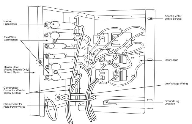
Fig. 10 - Fused Heater Control Box
