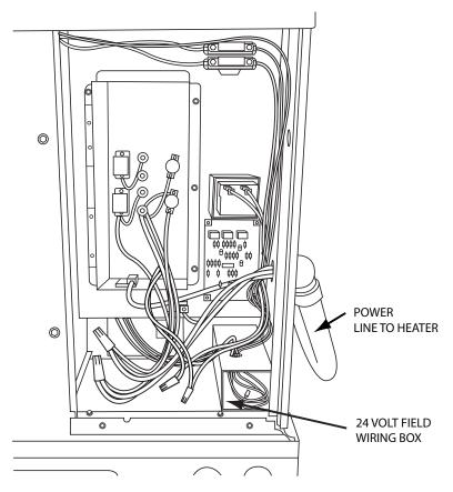
Fig. 7 - Single Point Connections for Non-Fused Heater
