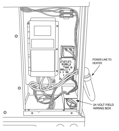
Fig. 6 - Single Point Connections for Fused Heater
