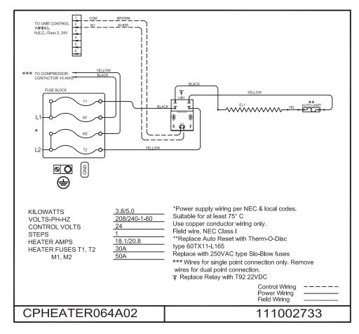
Fig. 26 - CPHEATER064A02 Wiring Diagram
