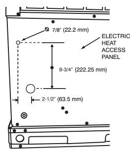
Fig. 2 - Second Power Line Access Hole Location
