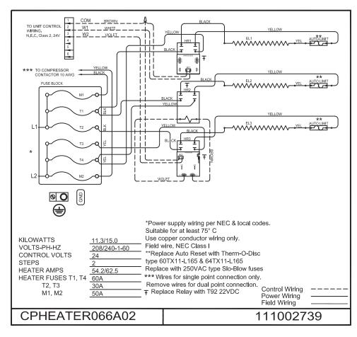
Fig. 28 - CPHEATER066A02 Wiring Diagram
