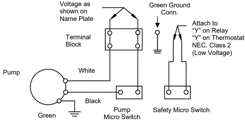
To test safety float switch, temporarily stop flow of discharge line by sharply bending vinyl tubing. Pour more water into pump inlet. Water level will rise beyond high level of control float until safety float switch breaks the "Y" thermostat circuit shutting down air conditioner condensing unit. Unbend the tube and the pump will empty the entire sump. Replace inlet line into pump inlet.
