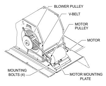
Fig. 70 — Belt Drive Motor Mounting
