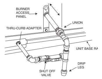
Fig. 32 — Gas Piping with Thru-Curb Accessory (Alternate Layout)
