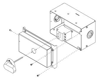
Fig. 46 — Handle and Shaft Assembly for NFD (Sizes 089-150)
