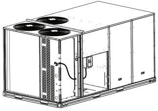
Fig. 39 — Conduit into Factory Option Disconnect
