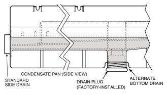
Fig. 35 — Condensate Drain Pan (Side View)
