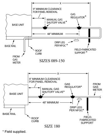
SPACING OF SUPPORTS X STEEL PIPE NOMINAL **DIAMETER** (in.) **DIMENSION (ft)**  $1/_{2}$ 6 <sup>3/</sup>4 or 1
