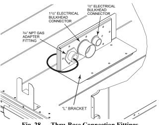
Fig. 28 — Thru-Base Connection Fittings (Size 180 Shown)
