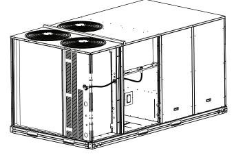
Fig. 40 — Conduit into Control Box
