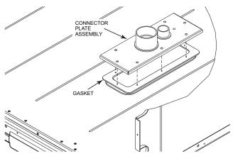
Fig. 56 — Completing Installation of Thru-the-Base Option
