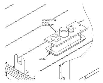
Fig. 29 — Completing Installation of Thru-the-Base Option (Size 180 Shown)
