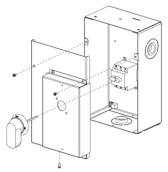
Fig. 47 — Handle and Shaft Assembly for NFD (Size 180)
