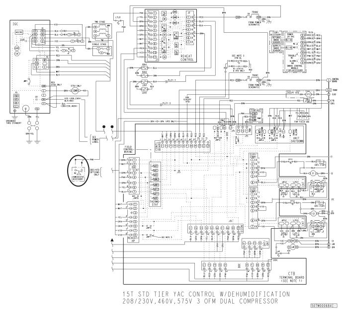
Fig. 59 — RGS180, Typical Hot Gas Re-Heat System Humidistat Wiring
