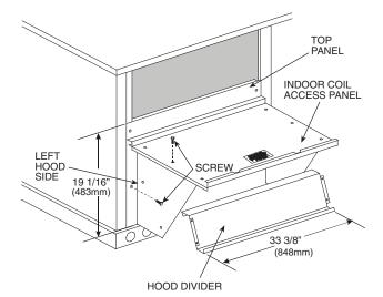
Fig. 18 — Economizer Hood Construction (Size 089-150 Shown)
