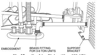
Fig. 27 — Gas Line Piping (Sizes 089-150)
