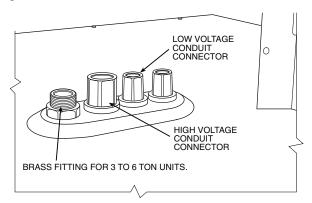
Fig. 26 — Thru-Base Connection Fittings
