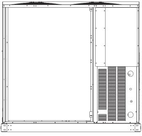
Fig. 41 — Mounting Position for Field Disconnects (over 100A)
