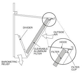
Fig. 19 — Economizer Filter Installation (Size 089-150 Shown)
