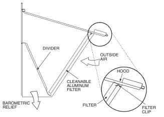
Fig. 22 — Economizer Filter Installation (Size 180 Shown)
