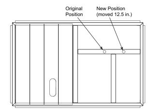
Fig. 12 — Alternative Condensate Drain Hole Positions
