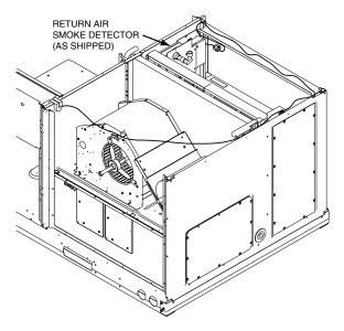
Fig. 66 — Return Air Smoke Detector; Shipping Position
