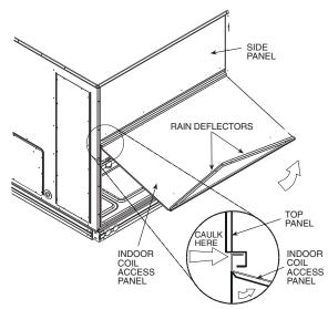
Fig. 20 — Indoor Coil Access Panel Relocation (Size 180 Shown)
