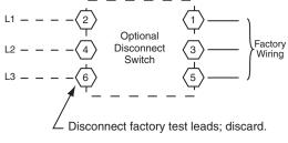
Fig. 38 — Power Wiring Connections (Sizes 180)
