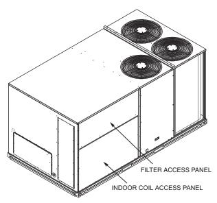
Fig. 14 — Typical Access Panel Locations (Size 180 Shown)
