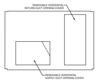
Fig. 13 — Horizontal Conversion Panels
