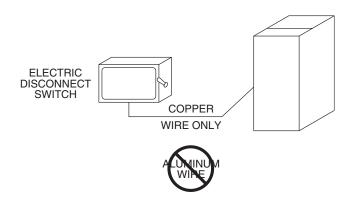
Fig. 43 — Disconnect Switch and Unit
