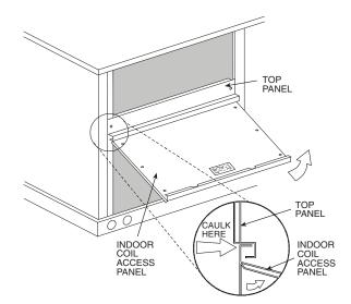
Fig. 17 — Indoor Coil Access Panel Relocation (Size 089-150 Shown)
