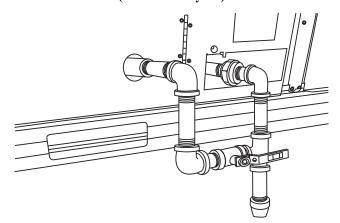
Fig. 33 — Gas Piping Thru-Base Connections
