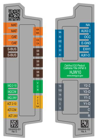
Fig. 61 — W7220 Wiring Terminals
