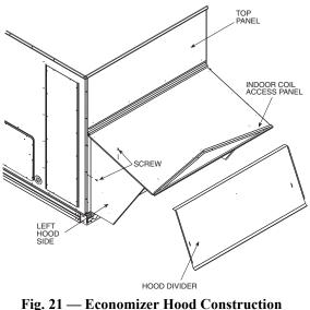
Fig. 21 — Economizer Hood Construction (Size 180 Shown)
