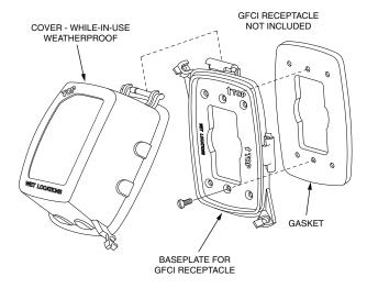
Fig. 50 — Weatherproof Cover Installation
