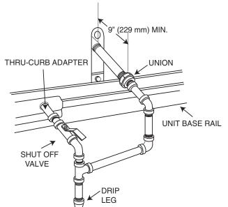
Fig. 31 — Gas Piping with Thru-Curb Accessory
