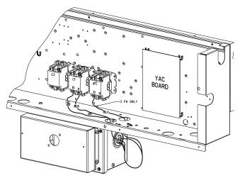
Fig. 44 — Location of Non-Fused Disconnect Enclosure (Sizes 089-150)
