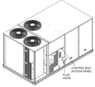
Fig. 24 — Flue Hood Details (Size 180)
