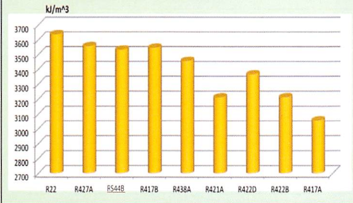
RS44B Capacity Evap temp 7°C & Cond temp +45°C
