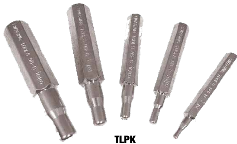
PRO-SET® SWAGE PUNCH SET 5 Punches (1/4", 5/16", 3/8", 1/2", 5/8")
