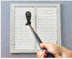
Attach the ABM-200, or TS-100 to the end of the EXP-64, to access hard-to-reach areas.
