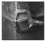
18. Compress gasket at corners with vice-grip while snapping in corner clips.
