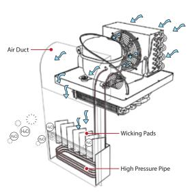
The new condensate chamber significantly reduces daily energy consumption thanks to yet another symbiotic design that re-uses energy. Surplus heat generated in the condensing unit is harnessed to evaporate overflow moisture collected in the condensate chamber. The air duct funnels hot air, the high pressure pipe channels hot gas, while the wicking pads speed up the evaporative process. All of these features come together for a system that is cost-effective in more ways than one.
