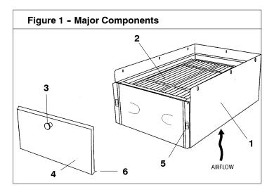
Introduction - These instructions cover the installation, operation and maintenance of an AHIC Fan Coil Media Air Cleaner.
