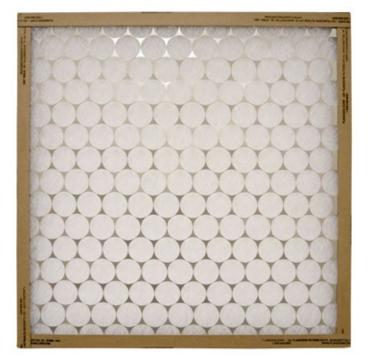
The Flanders Flat Panel EZ flow is a standard grade furnace filter of the same type that has been protecting furnaces and central air conditioners around the world for over 50 years. The filtering medium is continuous filament spun glass. The frame is made with one continuous piece of chipboard to guard against corner separation and is strengthened by a metal retainer. For peak equipment protection and energy efficiency, these filters should be changed monthly in periods of high use.
