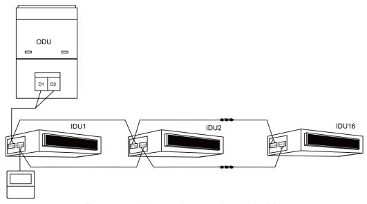
Fig.55 one wired controller controls multiple IDUs
