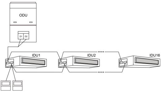
Fig.56 Two wired controllers control multiple IDUs
