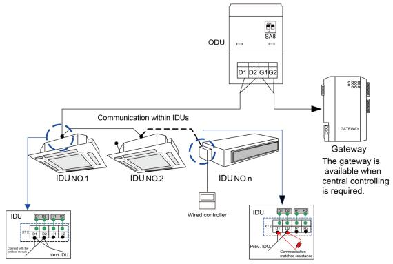
Fig.51 Connection of single unit
