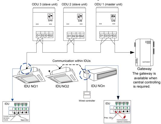
Fig.52 Connection of modular unit
