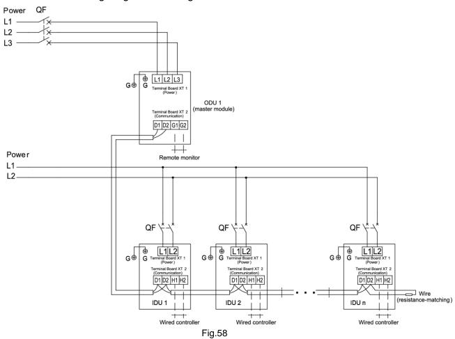
NOTICE! Maximum number of IDU is based upon ODU capacity. For details, please refer to the introduction of units' combination.
