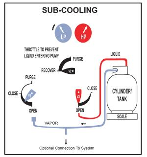
Figure 3-4 Setup Procedure for Sub-Cooling Method
