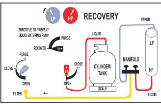
Figure 3-1 Setup Procedure For Normal Refrigerant Recovery
