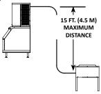
**15 ft. (4.5 m) Drop:** The maximum distance the Condenser or Condensing Unit can be below the ice machine.
