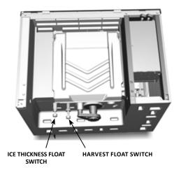
**Step 1** Disconnect power to the ice machine, remove the electrical panel to allow viewing of the control board lights. Disconnect the harvest float switch wire from the control board and place a jumper on the control board harvest switch terminals.
