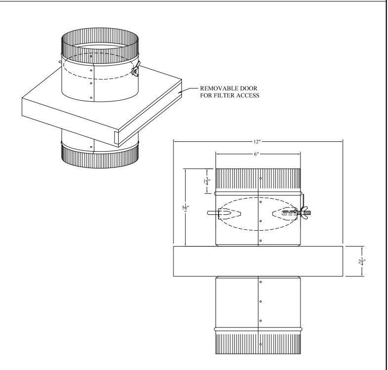
PART #: CP-ST1212INLINE | DESCRIPTION: 12X12 INLINE FILTER W/6" COLLARS AND DAMPER
