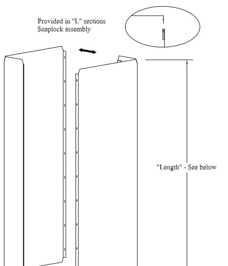
Corners notched for joint to joint or end cap assembly
