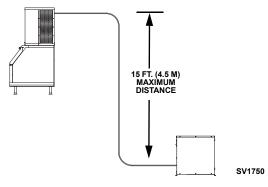
**15 ft. (4.5 m) Drop:** The maximum distance the CVD® Condensing Unit can be below the ice machine.
