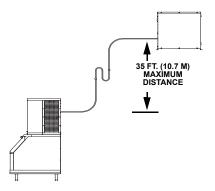
**35 ft. (10.7 m) Rise:** The maximum distance the CVD<sup>®</sup> Condensing Unit can be above the ice machine.
