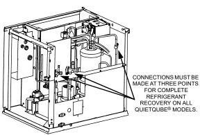
**Refrigerant Recovery Connections Ice Machine Head**
