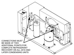
**Refrigerant Recovery Connections CVD Condensing Unit**
