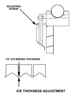
3. Make sure the ice thickness probe wire and bracket do not restrict movement of the probe.
