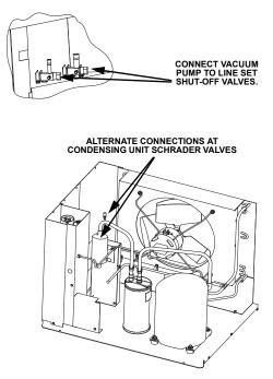
Isolate the vacuum pump from the line set shut-off valves and/or condensing unit access ports prior to proceeding.
