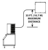
**35 ft. (10.7 m) Rise:** The maximum distance the Condenser or Condensing Unit can be above the ice machine.
