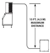
**15 ft. (4.5 m) Drop:** The maximum distance the Condenser or Condensing Unit can be below the ice machine.
