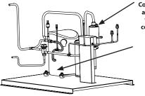
Connections must also be made at two points on condensing unit for complete refrigerant recovery.
