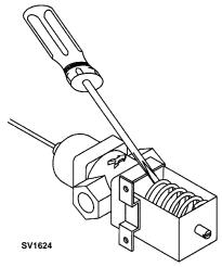
Hold the valve open and blow compressed air through the condenser until no water remains.
