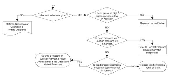
Single Evaporator Systems with Dual Harvest Valves: If one Harvest Vavle is open and the other is restricted / stuck closed you may have normal harvest pressures. Look for ice not melting on one side of the evaporator.
