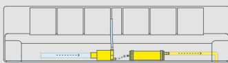
Water sensor and pump in the AC unit next to each other.
