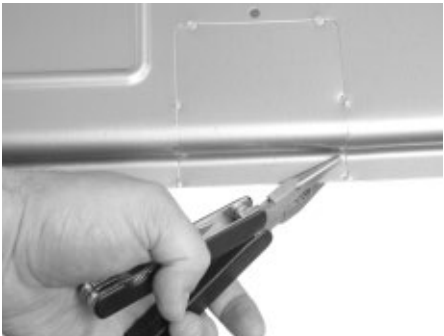
FIGURE 11 REMOVING CONDENSATE KNOCKOUT
