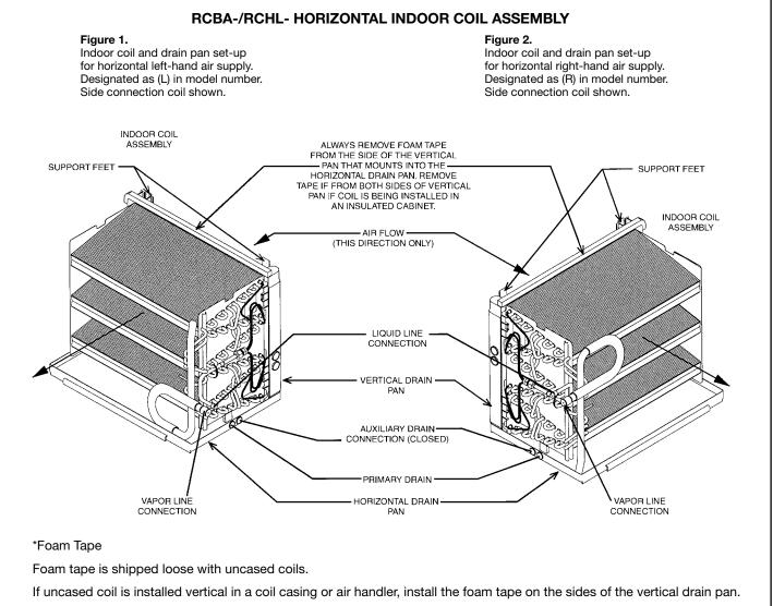
If installed horizontal, **DO NOT** install foam tape on the side of the vertical drain pan that fits into the horizontal drain pan. Remove foam tape, if already attached, from the side of the vertical drain pan that fits into the horizontal drain pan.
