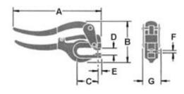
**CARE:** Oil at hinge points, the punch guide hole in the lower handle, and the punch point is all the care necessary.
