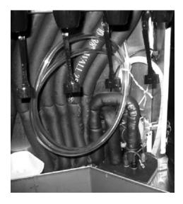
2. Purge tube is connected to the pressure relief valve on carbonator tank and must be routed to a drain. Route carbonator tank purge tube (A) down through the valve leads conduit, which is located behind the carbonator tank. Be sure not to collapse or kink carbonator tank purge tube during routing from unit to drain. 3. The carbonator tank purge tube (A) will be routed down through the valve leads conduit and out bottom of unit to a drain.
