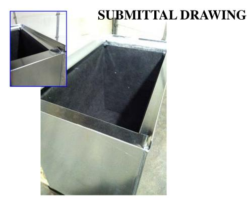
All 24 ga. galvanized metal. No rail on filter/door side. Removable rails on remaining sides. Available Lined (#929) or Unlined (#939). When ordering the first dimension should be non-rail side.
