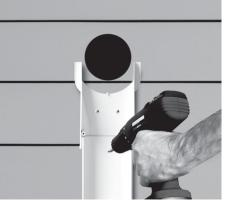
(2) Once all fitting bases are secured to the siding, measure and cut SD Ducting to fit as needed. Remember to account for some seasonal expansion and contraction. Install and fasten SD Ducting bases. Attach bases only to structure through provided punch outs using fasteners of sufficient length (not provided).
