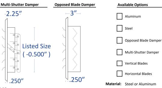
**Model Features** Two way air flow pattern Face: Adjustable curved blade Durable white powder coat finish Fin is encased in roll formed 22 gauge steel **Model Size:** Project Name: Architect:
